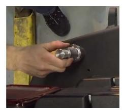
3. With the spindle in the bumper, install the lower 3/4" grade 8 bolt into the bottom of the spindle. You may need to lift the spindle a little to help get the bolt threaded. Once you have the bolt started use a 1 1/8" wrench to tighten the lower bolt.
