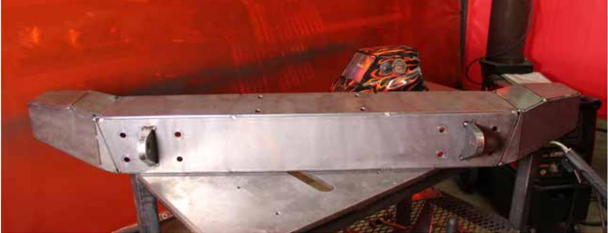
**17** Clamp the skid (Part #03) so that you can bend the top mounting tabs. Bend these to 35 degrees. The lower mount is bent the other direction to 42 degrees.
