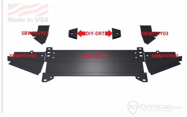
The first piece you will want to bend will be the (1) front Center Section. You will be bending two 90\* angles. It doesn't matter which side you make the front.
