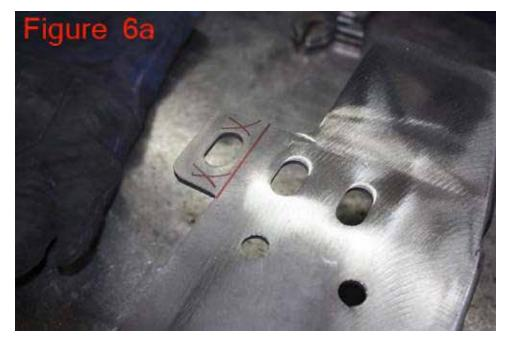
Mounting on a Jeep YJ. The lower tab will need to be trimmed to allow for clearance with the front leaf spring shackles. The area needing trimmed is pictured in Figure 6b.
