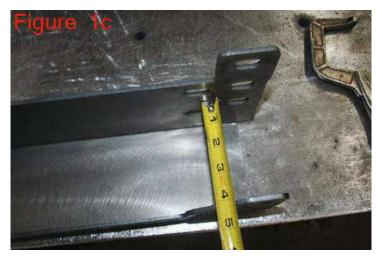
Each DIY Kit includes wings for a standard width bumper ( $\sim 51.5$  wide, Part 2) and stubby width ( $\sim 41.5$  wide, Part 3). If you are choosing to build a standard width bumper, follow the following steps. If you are choosing to build a stubby bumper, please advance to Step 4.
