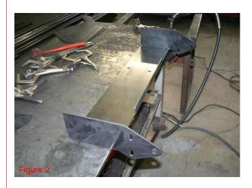
3 Set the bent Winch Plate (1) off to the side. Next you will need to bend the two Bumper Wings Both the top bend and bottom bend both will be bent to 90°.
