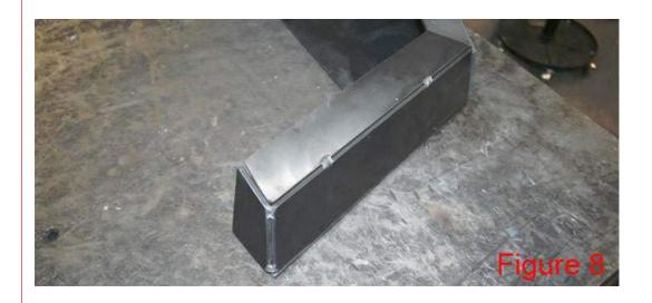
After every part is securely tacked , it would be wise to test fit the bumper on your Jeep before final welding, grinding, and finishing.
