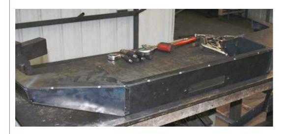
10 With the bumper tacked together and fit checked, it is now time to fully weld the bumper together. We recommend welding the back side first.
