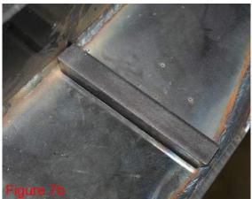
The Front Uniframe Reinforcement kit will need to be installed before installing the bumper. Without the additional plates, the bumper mounts will be too wide for the front factory frame rails. If you have your own or another brand of Uniframe tie in brackets, you will need to remove the front three bumper mounts in order to install the bumper.
