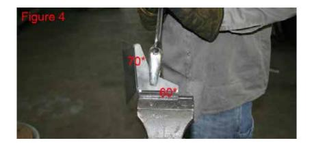
5 With all the bumper parts bent, the last thing to bend will be the rear bumper mounts. These mounts require four 90\* bends. \*\*\*You will need to bend a Right and Left, which will end up having two mounts that are opposites.\*\*\*
