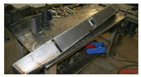
**10** After the bumper has cooled off some, this is where we recommending doing the grinding. You may want to do preliminary grinding here and finish grinding at the end, but the shell of the bumper is easier to grind before the dring tabs are welded in.
