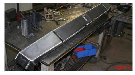
**11** After finish grinding the bumper, you can now install the under tail light caps (4). In order to get them to sit flush and correct, the bumper needs to be ground. After tacking each side into place, you will now fully weld them in place. Once you finish welding, grind the exposed welds.
