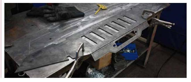
**2** Set the bent Center Section (01) off to the side. Next you will be bending the Winch Plate (04).
