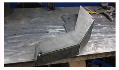
6 With the bumper tacked together, it is now time fully weld the bumper together. We recommend welding the back side first.
