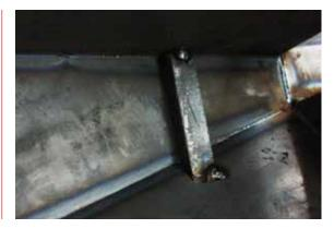
11 With the Dring Tabs (DRT) tacked into place, tack weld in the Bumper Mounts (05). You will notice that the mounting bracket will rest against the inside of the Dring Tab.
