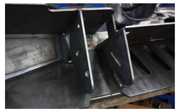
12 Make sure the Bumper Mounts (05) are square. The inside of brackets measurement from Driver side to Passenger side should be 32.5" It is best to leave the Dring Tabs and Mounts tacked into place until after test fitting the bumper on the Jeep.
