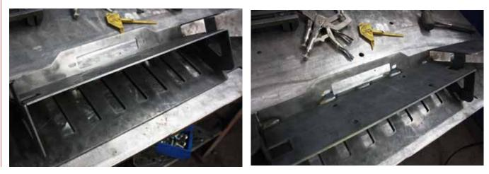
**9** Now that the entire bumper is tacked together, it's time to fully weld and grind the bumper!
