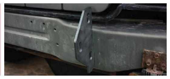
**18** On the ends of each side of the factory bulkhead are two pinch seams. These seams will need to be bent over before fitting the bumper. As shown with the red lines below, bend the lower seam underneath and the front seam over to the front.
