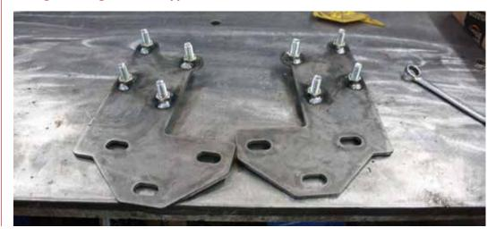
**14** Set the Frame Mounts off to the side and grab the Bulkhead Mounts (07).
