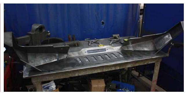
8 With the bumper still face down on the table, insert the Winch Plate (04). Assure proper fit and tack into place.
