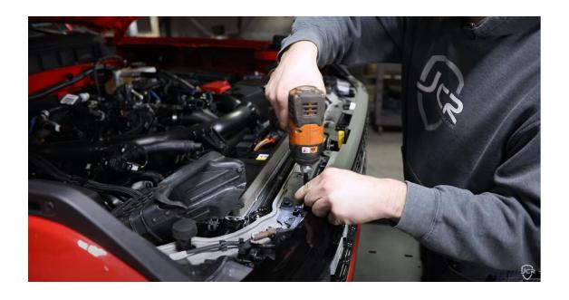
**3.** With the screws now removed, make sure to disconnect the coax cable for the front camera and the nozzle for the sprayer hose before removing the grille assembly.
