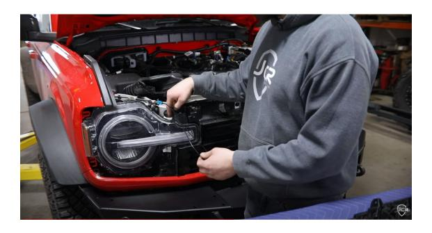
**9a.** Next you're gonna replace the factroy length of hose with the provided longer hose to route to the bumper. To do this, start by disconnecting the camera from hose so now you still have the male and female ends.
