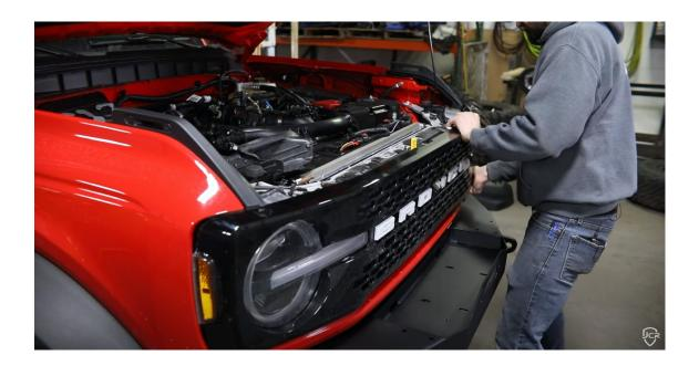
**5.** With the grille removed, remove all the clips holding the hose down, working from the outside to the center using a pry tool or flat head screw driver.
