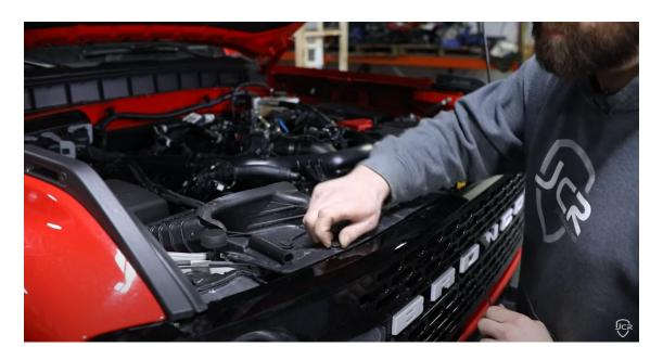
2. Next, behind the top grille remove the (4) factory mounting screws using a 10mm socket, as shown below.
