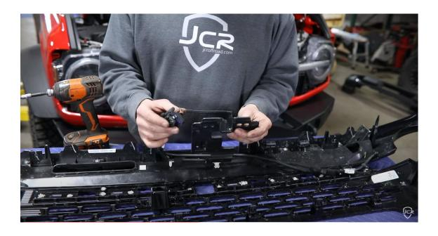
**8.** Before you reinstall the grille, you will need to route your provided cable extension down behind the headlight and out through the bottom in between the bumper, as shown below. With the cable now fed through, plug in the end and feed the excess cable down though the grille.
