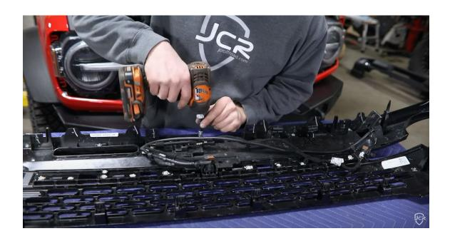
**7.** Once all (3) bolts are removed, you can remove the whole camera assembly and pop off the cover to the camera and remove the whole assembly from the bracket.
