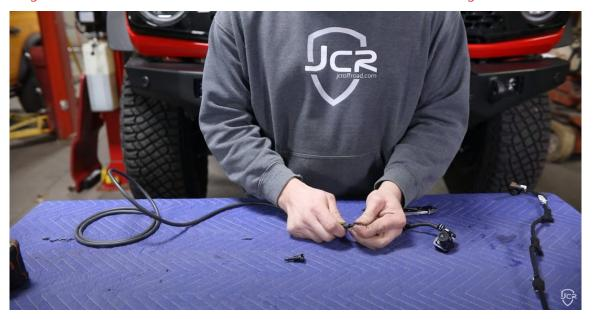
**10.** With the fittings now attached to each end of the hose, take the camera and connect it back to the male connector on the hose as shown below. You can now route and connect the opposite end back into the body from under the grille, leaving the camera end exposed to use on the bumper.
