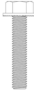
M8 x 1.25mm Thread, 40mm Long Hex Head
