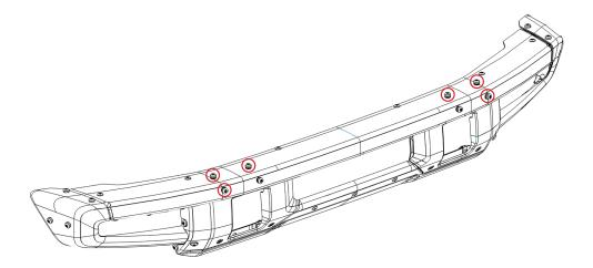
2 Once those are out of the way, place the tube onto the bumper and install it into the holes you just cleared using the factory bolts.
