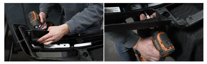
7 Next, push the three oval clips through the center bracket. Then, use the T40 torx bit to remove the two bolts holding the bracket in from the bottom as well as the three in the front of the bumper. Then you can remove that bracket.
