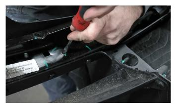
6 Next, use a T40 torx bit to remove the three bolts holding each bracket in from the top as well as the four holding them in from the bottom. Once those are out of the way you can remove the brackets.
