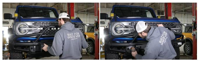
**15** Next, reinstall the plastic covers over the winch mounts using the factory clips.
