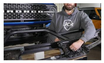
**4** Then next few steps are only for those who have proximity and parking sensor and wish to keep them while running the winch plate. If you do not, skip to step 13. First, remove the four bolts holding each of the large metal brackets behind the recovery points so that you can remove the brackets as well. Then, with those out of the way you can use a panel tool to pop all the clips holding the sensor wiring harness out.
