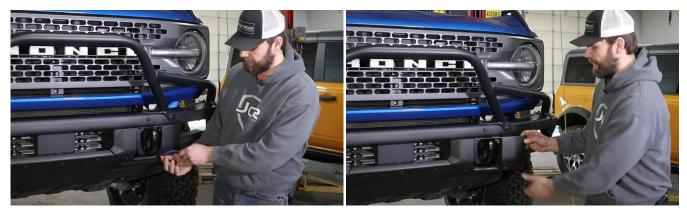
2 If your vehicle is equipped with parking and proximity sensors, you will need to locate the connector for that wiring harness and disconnect it. Then, use a 15mm socket to remove the three bolts holding the bumper in on each side. Be careful because they are the only things holding the bumper in place. Do not fully remove them until you are ready to pull the bumper off.
