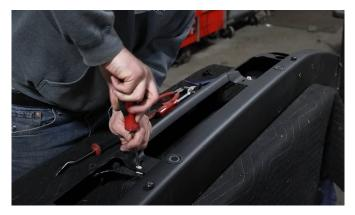
**9** With everything out of the way, you will need to remove the middle two sensors. To do so, apply pressure from the front with one hand while pulling the tabs on the top and bottom apart.
