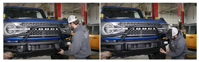
16 Finally, slide the winch plate back into place and install it using the 1/2" hex head bolts and washers on the outside with another 1/2" washer and a 1/2" nylock nut on the inside. This requires a 3/4" socket and wrench. If you have sensors, rout them up through the bottom of the winch plate and secure them in the provided holes with the provided rubber grommets. If not, insert the provided 1-1/4" plastic caps into them instead.
