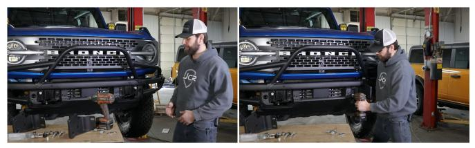
With both mounts loosely installed, slide the winch plate over the top of them and run one bolt through each side just to hold it in place for now. Then, center the bumper and winch plate on the vehicle and tighten the mounts fully into place. Then, remove the winch plate for now.
