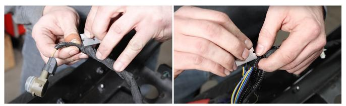
Once you are done, it should look like the image below. At this point you will need to re-tape the harness as well as the newly exposed wires with electrical tape in order to make sure no wires remain exposed.
