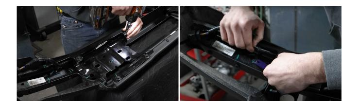
**5** Next, push the oval clips in from the back of the metal brackets that the sensors were attached to.
