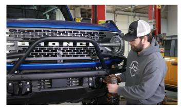
**3** With the bumper off of the vehicle, use a 10mm socket to remove the small bolt in the middle of each of the metal brackets behind the recovery points. You can then pull the recovery points off.
