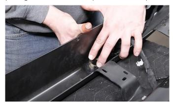
**10** Next, use wire cutters to carefully remove the two clips that are just past the sensor as you move towards the middle on each side.
