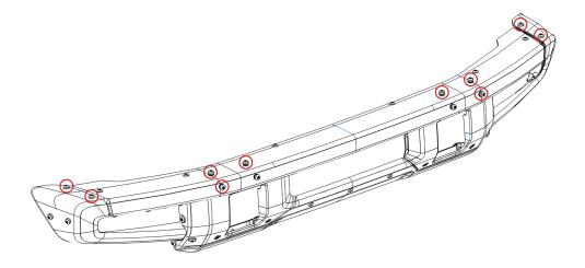
Once those are out of the way, place the tube onto the bumper and install it into the holes you just cleared using the provided M8 bolts. The easiest way to do this is to start with the center bolts and work your way out. That way it is much simpler to line up each end. If you are sill struggling to get everything lined up, you can adjust the position of the caps on either end of the bumper as well.
