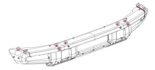
2 Once those are out of the way, place the tube onto the bumper and install it into the holes you just cleared using the provided M8 bolts. The easiest way to do this is to start with the center bolts and work your way out. That way it is much simpler to line up each end. If you are sill struggling to get everything lined up, you can adjust the position of the caps on either end of the bumper as well.
