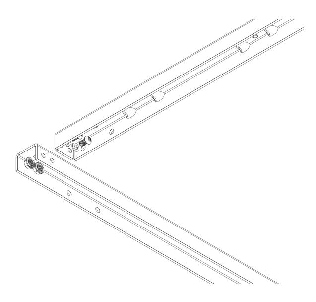
2. Once the (2) side brackets are assembled and tight to the front, you're going to install the (4) provided corner support brackets. These install using the provided 1/4" button heads, washers and flange nuts. Be sure to assemble in the correct orientation as shown below, with the back flange going on the inside of the front bracket and the inside flange on the outside of the side brackets.
