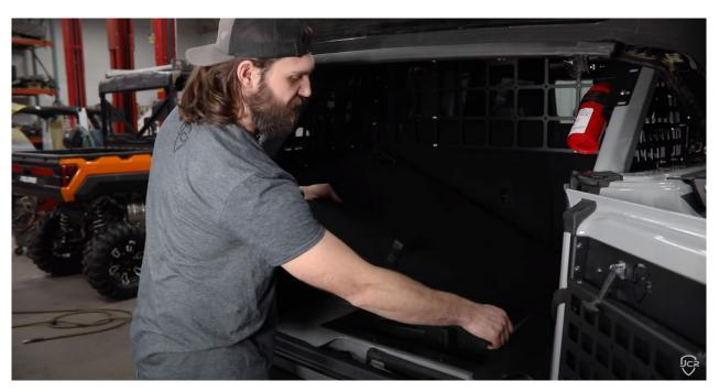
**5.** With the factory floor now out of the way, you can grab the frame you assembled and place it in the back of the Bronco. Be sure to make sure that the teardrop cut outs in the middle bracket are away from you, going in toward the front of the vehicle. You may have to insert the frame at an angle to get it to fit into the back. Once it is in the vehicle, lay it flat and push forward and down and it should kind of snap into place between the plastics.
