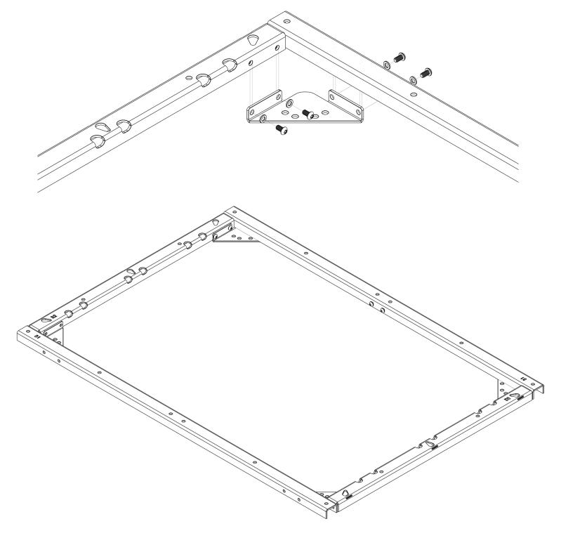
**3.** With the (4) outside brackets assembled and tight with the corner supports, you can install the provided middle bracket using the 1/4" button heads, washers and flange nuts. This will install pretty much the same as the side brackets to the front and back brackets. Be sure to install in the orientation below with those teardrop cut outs at the top pointing out and down toward the middle. Be sure to do this on both ends of the bracket.
