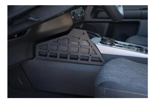
2 Make a hole in the center console at each mark using either a 1/8" drill bit, or a pick. Only drill deep enough to get the screws started, it is not necessary to drill all the way through. This will prevent any possibility of damaging anything behind the console. Then, install the panel using a Phillips screwdriver. Use 1 screw and 1 spacer per hole.
