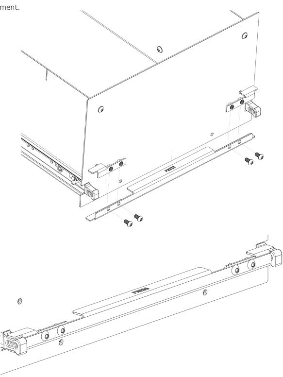
**10.** The final step is to secure the handle cover bracket to the front of the drawer to complete your install. Take (4) of the provided 1/4" button heads, washers and flange nuts and use them to secure the bracket to the panel, as shown in the orientation below. \*If you've purchased our label kit, you will install them here before securing the handle cover.
