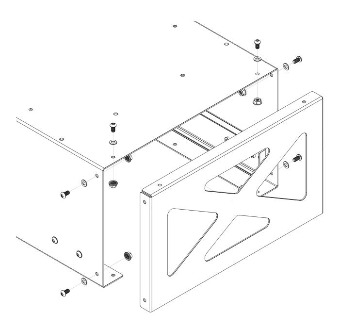
**3.** \*This step only applies to 10" drawers. Next, mount the (2) provided L shaped brackets in the upper inside corners of the slide assembly with the provided 1/4" button heads, washers and flange nuts as shown in the orientation below. Make sure to do this on each side.
