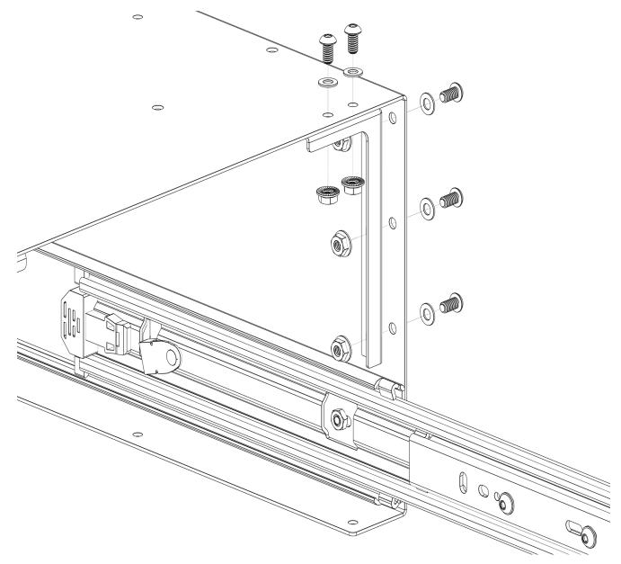
**4.** Once you have all of that assembled, you can now bolt the cabinet assembly to your floor through the (4) bottom mounting holes on each side using the provided 1/4" button heads, washers to secure into nutstrips. For more details on our vehicle specific floor systems, be sure to check out our product page on our website and watch our install video.
