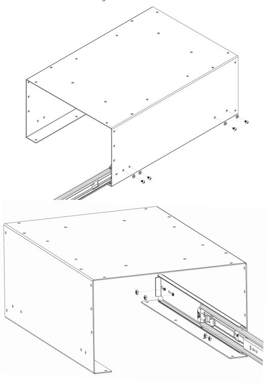
2. Next, take the back piece of the cabinet assembly with the "X" cutout and bolt that piece to the main U shaped slide piece using (6) each of the provided longer 1/4" button heads, washers and flange nuts as shown in the orientation below.
