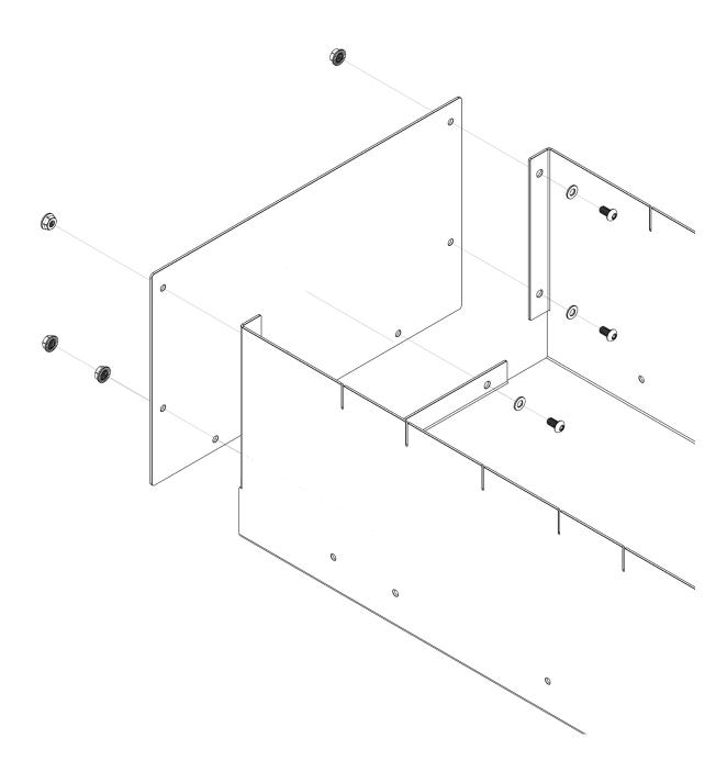
**6.** Once the back piece to the drawer is attatched, you can now slide in the provided divider piece from the top into whichever slot in the drawer to your liking, as shown below. Edge trim will be provided to be cut and trimmed to nest inside the cutouts of this panel.
