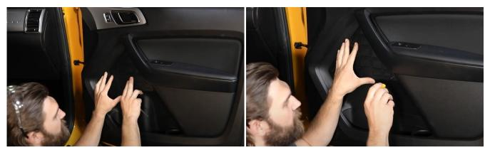
2 Once all the holes are marked, set the panel down and make a hole in the door plastic at each of the marks. This can be done using a 1/16" drill bit, or we have had luck simply pushing the sharp punch tool through the plastic. Whatever you decide to do, be careful not to make the holes to big or to go to deep. Going too deep could potentially lead to you hitting something important withing the door such as wiring.
