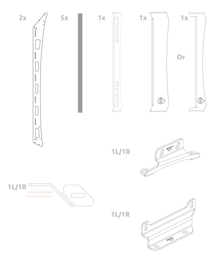
Assemble the rack on the ground. Start by mounting the crossbars between the two side rails. For this, use the 1/4"-20 X 3/4" button head bolts and the 1/4" ID washers (2 per bar per side). Make sure the machined slot in the rail of the crossbar is facing up, so that you can easily add t-nuts to mount your gear.
