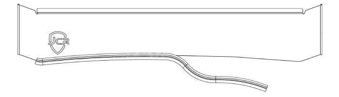
**3** Mount the front and rear fairings. To do this, use the 1/4"-20 X 3/4" button head bolts, 1/4" ID washers, and 1/4"-20 serrated flange nuts. The front fairing will need 3 of each per side and the rear fairing will need 2 of each per side. When mounting the fairings, adjust them all the way up and tighten to avoid contact with the roof when setting it in place.
