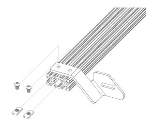
2 Next, place your light bar between the mounts and mount it in the slots using the hardware provided with the light bar. After that is firmly in position, make any adjustments to the positioning necessary to center the light bar on the rack. Depending on the rack and light bar, you may need to adjust the position of the cross bar in its slot as well.
