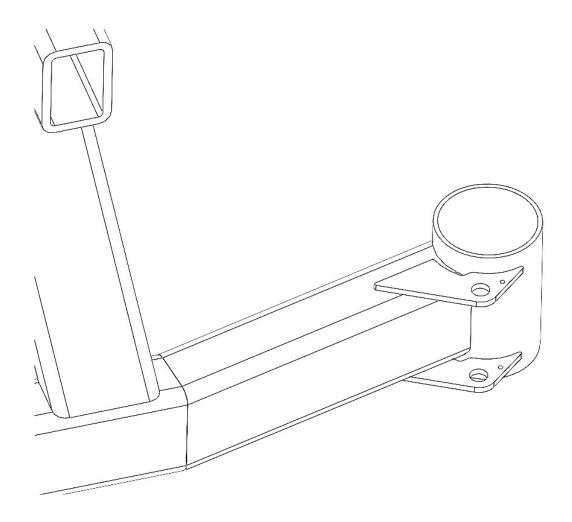
**5.** You can now take the top tube support bracket and the spare tire mount bracket and weld them to the top tube, as shown in the orientation below. There will be an etching that matches the profile of the tube on the spare tire mount that will line up, once aligned weld the faces flush. Then make sure the tube supprt bracket will line up in the middle of the top tube and flush on the base of the "A" shape tube before welding into place.
