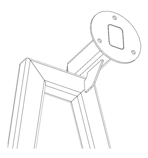
**6.** You can now choose to mount and weld the supplied High Lift mount to the carrier if you please. Take the offroad jack mount bracket and line the small top flange flush with the top tube face, and the larger bottom flange should sit flush with the bottom tube, as shown in the orientation below (viewing from the back side). And once you have all three sides of the bracket flush with the tube, weld the bracket into place.
