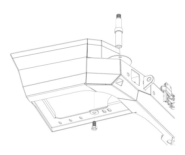
**10.** Next, grease both bearings and the rubber seal. For more in-depth instructions on how to do so, watch the installation video. Then, flip your carrier door upside down, and insert 1 bearing and the rubber seal into the hub. Make sure that in this orientation, the smaller end of the bearing is facing down, and the softer rubber lip of the seal is facing up. You will then need to tap the seal into place using something such as a hammer and screwdriver.
