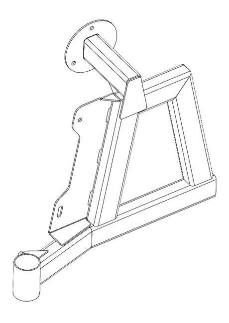
**7.** Take the (3) provided tie in brackets and weld them onto the frame for added strength. The first (1) one will be an oval shaped piece that will mount over the lower angled tubes on the front and backside. The second (2) and third (3) pieces will mount flush with the backside of the tubes in the top and bottom corners, as shown in the orientation below. Once your brackets are all in place, fully weld them down.
