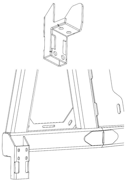
**9.** Next, install the spindle into the bumper. Put the larger end of the spindle into the hole on the pin track. Then, use the 3/4" x 1-1/2" bolt with the 3/4" washer to secure it onto place. To do this you will need to insert the bolt and washer into the threaded hole in the bottom of the spindle by reaching around to the back of the bumper from the bottom.
