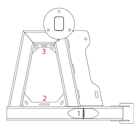
8. Now, take all of your latch bracket pieces and bend them all on the bend lines 90 degress. Once bent, weld them together as shown in the orientation below. There will be tabs on the smaller piece to line up to with the larger one. Once those are welded together, take that assembly and weld it onto the end of the bottom tube (also shown below). Note that we are showing right side carrier and latch orientation, you will have to mirror this operation for a left side.
