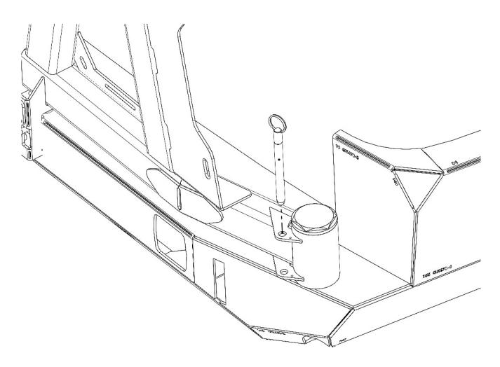
**14.** Next, open the carrier as far as your tire will allow before hitting the vehicle and drill a hole into the top face of the bumper with a 1/2" drill. This will be the stopping point for the drop pin and carrier.
