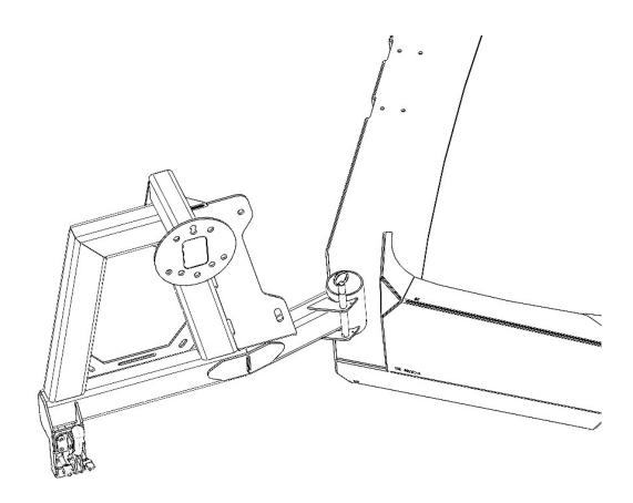
**15.** If you are happy with the look and alignment, you can now go though and fully weld the carrier to finish the assembly. You are now finished assembling your DIY carrier. At this time you are free to customize and set up the carrier to your liking, as you can see from the picture below there are different ways you can set up and run your carrier. Also be sure to check out JCROffroad.com for our DIY bumpers and other XJ product.
