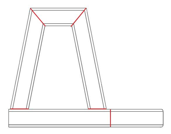
**3.** Now that base tube work is welded together, take the last piece of provided tube and the the #3 bracket and weld them both together to the rest of the base, as shown below (view from the back of the carrier). Be sure the profile of the bracket and the tube match up before welding into place. This can also be moved side to side to best fit your needs and tire size.
