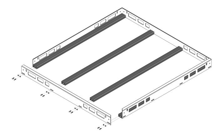
5 Next, attach the floor panels to the tops of the cross bars. To do this, place a panel onto the bars so that it is perpendicular to the direction of them. Then, slide the T-nuts into position so that they are beneath the holes in the panel. After that, bolt them together using the 1/4"-20 X 3/8" bolts and 1/4" washers. You may need to slide the bars around to line the holes up as well. Once the floor panels are all in place, go back around and tighten all the bolts you left loose earlier.
