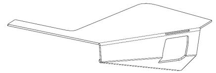
2. Before fullying welding the heavily tack pieces together, we reccomend you solidly tack the majority of these parts together incase you need to adjust or change anything. Take the (4) provided pieces as shown below, and weld them into the formation shown, aligning the profiles and angles to one another. Also be sure to leave a gap as shown below to add in the D-rings later. Weld the seams and make sure everything is level and square.
