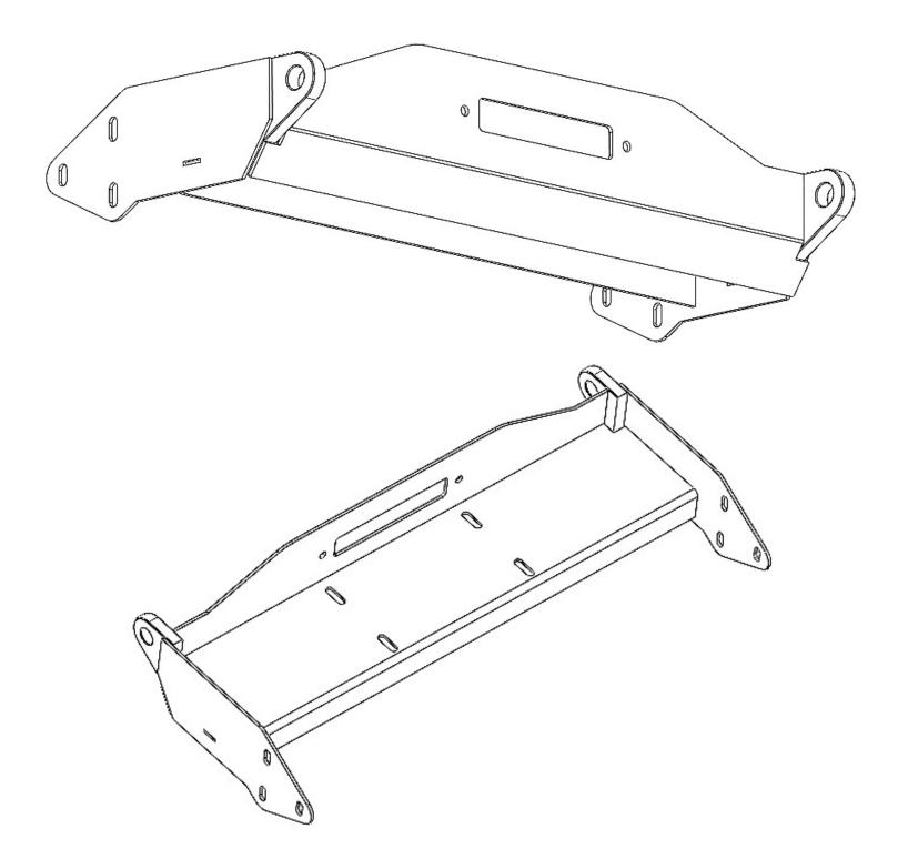
**4a.** Once the D-rings are welded into place on the base, take the (2) supplied wing pieces for each side brackets and weld them onto the center section (as shown below), with the top face flush over the D-rings and nesting in the corner before it jogs up. The outside wing piece should nest and fit right into the other as long as the angles are correct. Once both wings are tacked on, you can loosely bolt it onto the truck to check alignment.
