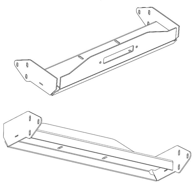
**3.** Now that the main piece is tacked together, it is now a good time to weld in the provided D-rings into place, as shown below. Be sure the back face of the D-ring is square to the cut out in the winch plate and the top face is level with the center section top face.
