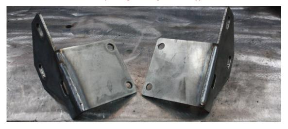
15 In order to install the Frame Mounts (06), you will need to open up the front oval holes in the factory bulkhead.
