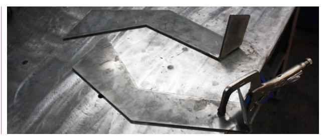
With all of the Bumper Parts Bent, it's time to start tacking things together!
