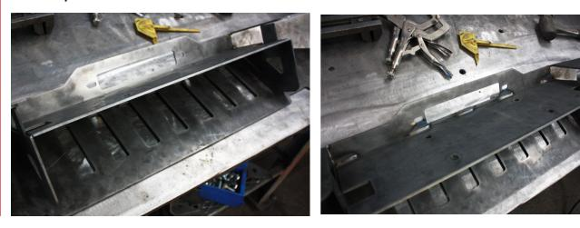
**9** Now that the entire bumper is tacked together, it's time to fully weld and grind the bumper!
