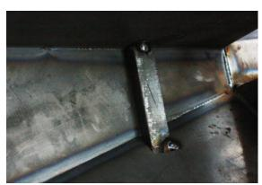
With the Dring Tabs (DRT) tacked into place, tack weld in the Bumper Mounts (05). You will notice that the mounting bracket will rest against the inside of the Dring Tab.
