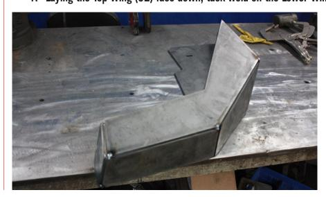
6 With the bumper tacked together, it is now time fully weld the bumper together. We recommend welding the back side first.
