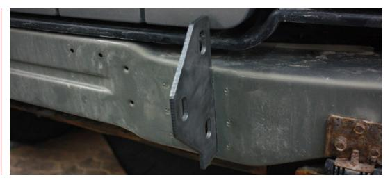
17 At this time you can bolt the Bulkhead Mounts (8) into place and drill the holes needed to mount them to the front bulkhead assembly.
