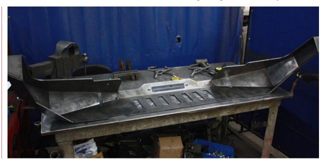
With the bumper still face down on the table, insert the Winch Plate (04). Assure proper fit and tack into place.
