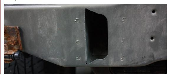
$16 \quad \text{Tests fit the mounts and trim more where necessary}.$
