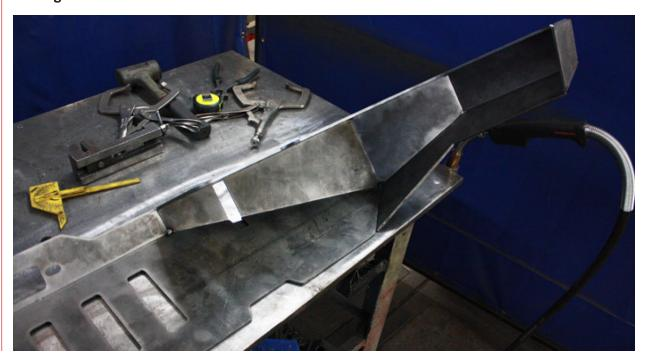
7 Shown below is the Center Section (01) with both left and right wings tack welded in place.
