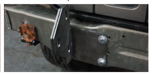
On the ends of each side of the factory bulkhead are two pinch seams. These seams will need to be bent over before fitting the bumper. As shown with the red lines below, bend the lower seam underneath and the front seam over to the front.
