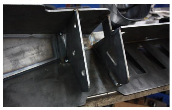
Make sure the Bumper Mounts (05) are square. The inside of brackets measurement from Driver side to Passenger side should be 32.5" It is best to leave the Dring Tabs and Mounts tacked into place until after test fitting the bumper on the Jeep.
