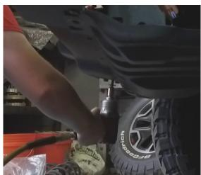
After you remove the lower skid plate, remove the front bumper from the frame rails by unbolting the 4 bolts on each side.
