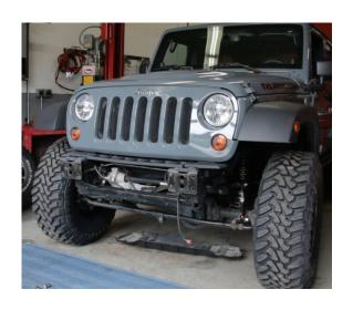
Remove the plastic cover panel on top of the frame. You can easily drill through the plastic screws if they spin in place.
