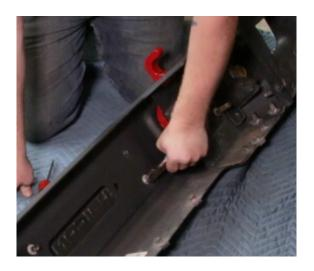
Most new winches utilize a "centered" style fairlead opening. These will use the centered fairlead plate. Others such as the Warn 9.5 CTI are offset and will use the offset fairlead plate. While the bumper is off, bolt your fairlead plate to the front. This is also a great time to install your JCR Fairlead!
