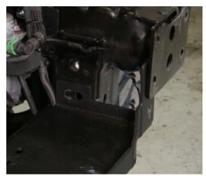
Raise the winch plate in to place so that the the side mounting points line up with the flag tab.
