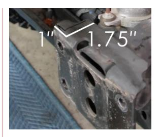
**5** Remove the vacuum pump using a 10mm wrench and rotate the pump 90 counter clockwise.
