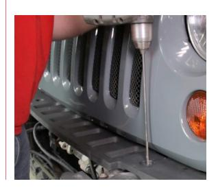
4 If you are using a larger winch, such as a Warn Zeon series, notch the front of the frame rail. The cut will need to be 1" wide to the end of the frame rail.
