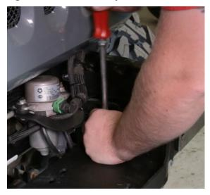
8 Install the winch to the winch tray and run your wiring into the engine bay
