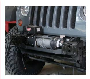
9 Using snips or wire cutters, cut the rubber stops on the back of the fairlead cover plate, discard of the plate as you will not be needing it.
