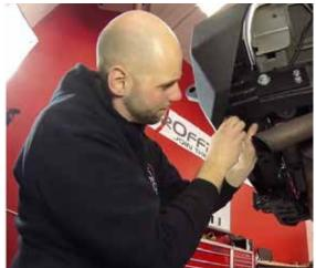
Next, using a 1/2 drill bit, drill a hole into the passenger lower mounting hole into the lower cross member. Once this is done, loosely install the two (2) half inch bolts into the lower cross member.
