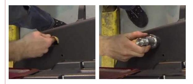
**3** With the spindle in the bumper, install the lower 3/4" grade 8 bolt into the bottom of the spindle. You may need to lift the spindle a little to help get the bolt threaded. Once you have the bolt started use a 1 1/8" wrench to tighten the lower bolt.
