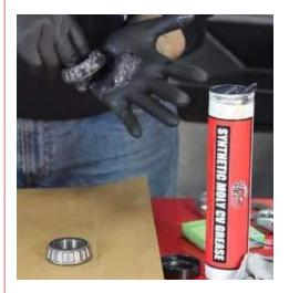
**5** Prop the carrier so you can install the lower bearing. Place the lower bearing tapper side down into the carrier. Using a large socket or a punch, knock in the lower oil seal with the green side of the seal going into the carrier. Make sure you hammer it in carefully and most importantly, straight. Now with the lower bearing installed, slide the carrier onto the spindle.
