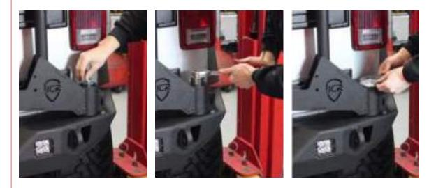
Using spacers provided, install the tailgate link onto the shield carrier with the 1/2" x 2" bolts and
