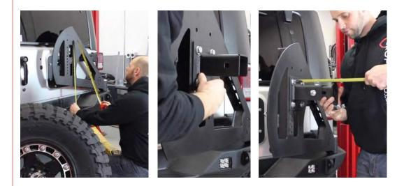
**9** Lengthen the tailgate link, then close the gate and install the 1/2" x2 bolt. You may need to use a punch to line everything up. Tighten the link until the rubber isolators touch the tailgate plate. Note that the rubber isolators may need to be shimmed out using washers. This all depends on how the bumper is positioned. Once adjusted, open the gate and tighten the jam nuts on the link.
