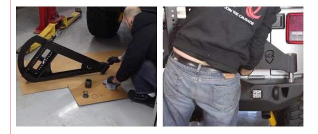
**6** With the upper tire carrier on the spindle, place the top bearing, tapper down over the spindle and into the hub. Next Install the large washer and top spindle nut. Using a 1 1/2" socket and snug it up (65 pounds). It may be necessary to place a wrench on the bottom bolts to achieve torque. With that tightened down, Install the o-ring onto the aluminum top cap and use the provide wrench to snug up the cap.ith the carrier on the Jeep.
