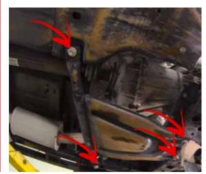
4 Continuing with the 18mm socket, remove the two factory fuel tank skid bolts in the crossmember.
