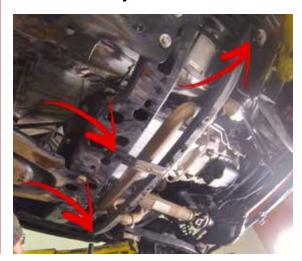
3 Still using the 18mm socket remove the four bolts holding the transfer case skid, if installed.
