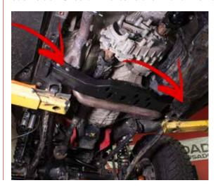
Remove the jack stand holding the transfer case and transmission up and let the transmission rest on the new crossmember. Thread the 16mm bolts back through the crossmember and into the transmission mount. Use the 16mm socket through the crossmember to tighten down those bolts.
