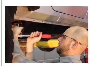
4 With help from a friend, porition the slider into place and loosly install the outer body mounts. If working on a 4 door JK do not install the middle body mount bolt just yet.
