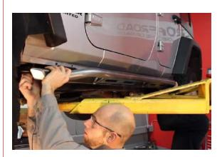
If working on a 4 door, hold the slider up against the pinch seam and install the 6 button head bolts and nuts. If working with a 2 door JK, you will install 4 of the button head bolts and nuts on each side. Once they are all in place, use a 3/16" Allen head wrench or socket, and a 1/2 wrench to tighten down all the bolts.
