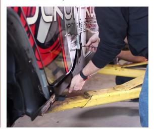
$10\,\,$  Tap the 6 clip nuts onto the inner panel outrigger mounts
