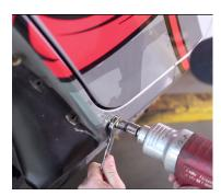
4 Temporarily install the inner panel using a 3/16" Allen and the 3/4" long stainless button head bolts. Use this inner panel as a template to mark out the rest of the holes. Make that the inner panels is flush against the body when you mark for proper hole placement. You can do this by drilling right through the slider, or by marking the holes with a marker and removing the inner panel. Either way, start with the 5/16 drill bit.
