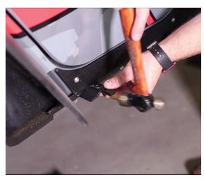
11 Using an 18mm, remove the lower body mount bolts.
