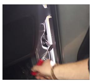
Grab the drill and 17/32 drill bit again. Enlarge the holes you just drilled now. In the front you are going to want to pull the loosened fender panel towards you while drilling. Note, that you will be drilling through two or three layers of sheet metal so take your time. Once all the holes are drilled, its a good idea to finish them with some spray paint to help prevent rust.
