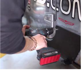
Remove the inner panels. Using a 10mm socket remove the front two pinch seam bolts. Also loosen the two fender bolts inside the door frame.
