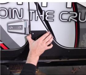
Pre-drill the two marked holes up to a 1/2 inch. Then using the 17/32 drill bit, drill the holes to the proper size for the nutserts. Be careful not to tear the sheet metal when doing this.
