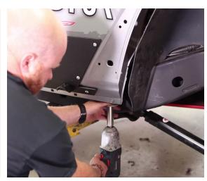
12 Install the LED lights using the provided button head bolts, washers, and lock nuts. Make sure the lights are centered in the hole and tighten them down using a 3mm allen and a 5/16" socket or wrench.
