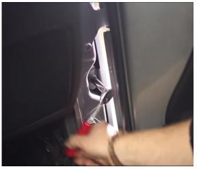
Apply anti-seize on all the 3/4" long stainless button head bolts and loosely install all 18 bolts that hold on the inner panel. Once all the bolts are installed, you can tighten them all up.
