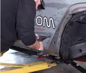
Using the provided nutsert tool, install the nutsert into the two holes you just drilled. We recommend you apply some RTV on the nutserts before installing them into the holes to lessen the chance of rust. For the nutsert tool use a 1/2 inch socket and a 11/16 end wrench. We recommend using an impact for speed, but it can be done with just hand tools. Go until the nutsert is fully crushed at 40 foot pounds.
