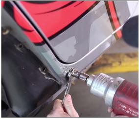
**8** Tighten the two lower fender bolts at the pinch seam and tighten the bolts inside of the door jam.
