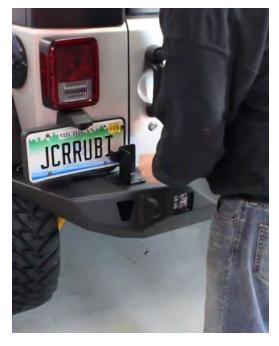
1. Start by installing the latch mount with the provided button head bolts onto the bumper.
