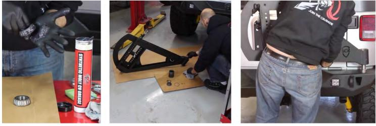
7. With the upper tire carrier on the spindle, place the top bearing, tapper down over the spindle and into the hub. Next Install the large washer and top spindle nut. Using a 1 1/2" socket and snug it up. With that tightened down, Install the o-ring onto the aluminum top cap and use the provide wrench to snug up the cap.ith the carrier on the Jeep.
