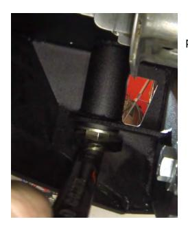
4. Next, Install the stainless plunger track onto the passenger side using the provided hardware.
