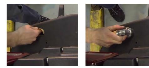
3. With the spindle in the bumper, install the lower 3/4" grade 8 bolt into the bottom of the spindle. You may need to lift the spindle a little to help get the bolt threaded. Once you have the bolt started use a 1 1/8" wrench to tighten the lower bolt.
