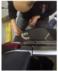
5. Next, pack the bearings with grease. Working the bearings around in your hands, knead the grease into each of the bearings. Apply a little grease to the inside of the oil seal as well as the top cap o-ring.
