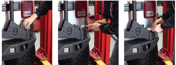
8. Install the plunger into the threaded mount next to the hub assembly. Install the latch with a 3/8" socket using the self tapping bolts. Using a 13mm wrench, you can adjust the latch to the desired tension.
