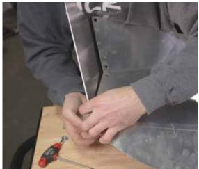
4 If you have NOT purchased our front fenders, you will need to do the following steps. Remove the wire loom (picture A) from the bolt hole (picture B) then open up the bolt hole to a 5/16". You will also need to open up the bottom bolt hole to a 5/16".
