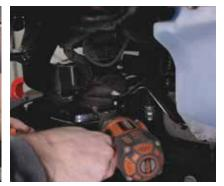
After you drill the hole, you can reinstall the inner fender.
