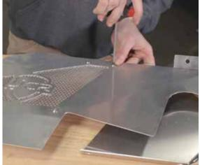
Next, install the other 2 panels on the opposite side of the main panel. Use the 5/16" button head bolts to secure these 2 small panels to the main panel. The triangle panel will be mounted underneath the main panel using 2 bolts, while the other panel will be mounted on the side of the main panel using 4 bolts. Use a 3/16" allen to tighten the bolts.
