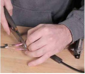
Once you connect all the wires, use a heat gun to secure the wires into the butt connectors. Use electrical tape to keep the wires connected and out of the way.
