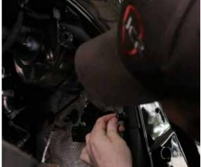
Once you remove the wiring clips, open up the bottom hole to a 5/16" with a 5/16" drill bit.
