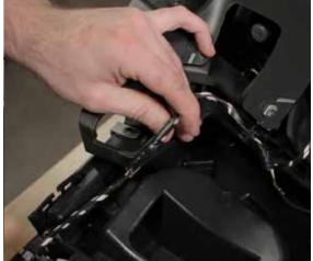
Next we will assemble the new fender. Start with mounting the LED light on the LED bracket. Run the 2 wires through the center hole. Use 2 1"-8/32" bolts to mount the light to the bracket. Use a 3/32" allen wrench and a 9mm open end wrench to tighten the bolts. Use 2 1/2"- 10/24" bolts to secure the LED light to the fender with 2 flange nuts. Use a 1/8" allen to tighten the 2 1/2" bolts.
