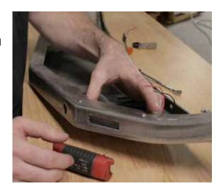
Mount the 3/4" LED light. Make sure the mount bracket loop faces the front of the fender. Insert the gromite into the loop then push the LED light through the gromite. Use 1/2"-10/24" bolts to secure the bracket to the fender. Use a 1/8" allen to tighten these bolts.
