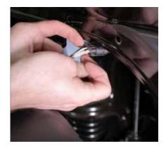
After you remove the fender, use your dash tool to move any clips that remain. Remove the factory vent panel by squeezing on the clips behind the panel and pry it out. Remove the plastic panel that was connected to the bottom of the fender by simply pulling on it.
