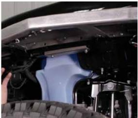
Next, install 2 5/16" bolts into the standoffs coming off the jeep into the upper brackets. Maker sure you use the round hole to install these bolts.
