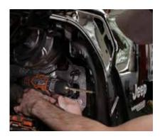
Temporarily install the fender support bracket lining up the 3 holes. Use a 3/16" allen to tighten the bolts.
