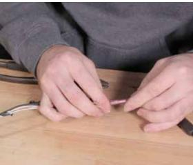
Connect the red wire from the running light to the white wire with the orange tracer coming off the factory harness. Connect the black wire from the daytime running light to the white wire with the brown tracer from the factory harness. Last, connect the red wire from the 3/4" LED to the white wire with the green tracer from the factory harness.
