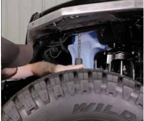
After you open the 2 holes up to a 17/32", install rivnuts. Check out our video on youtube to learn more about installing rivnuts. After you install the rivnuts, you can reinstall the bracket starting with the rivnuts. Only thread them half way then install the upper bolts sing the 1"-5/16" bolts. Go back and tighten down all of your bolts.
