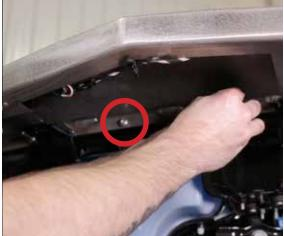
With the bracket installed, drill 5/16" holes into the crossmember through the 2 holes of the bracket. Once you drill the 2 holes, remove the bracket and open the holes we just drilled to a 17/32".
