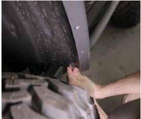
Disconnect the clips holding the inner fender onto the fender by simply pull upward on the edge of the fender, then set the inner fender aside. Remove the 4 bolts on the inside of the fender as well as the plastic retainers that hold the fender to the body of the jeep.
