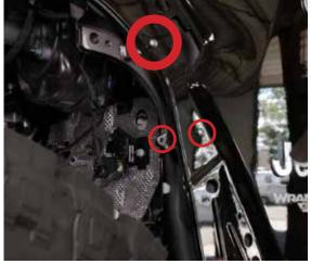
With the temporary bracket installed, drill out the right hole to a 5/16". Once you drill the hole, you can remove the 2 bolts on the surface of the body so we can install the fender.
