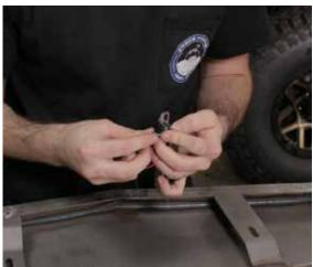
Use 2 1/2"- 10/24" bolts to secure the LED light to the fender with 2 flange nuts. Use a 1/8" allen to tighten the 2 1/2" bolts.
