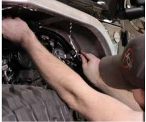
Install the rest of the bolts except for the top 2 holes on the fender. Leave those empty for now so we can install the 2nd bracket later.
