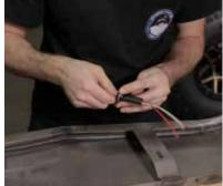
Next we will wire the fender. Connect the black wire from the running light to the white wire on the 3/4" LED then put a butt connector on. Connect the other end of the butt connector to the black wire coming off the factory harness.
