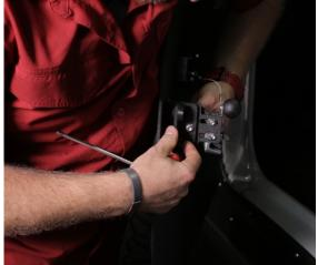
Last we will secure the doors to the jeep using nylock's to go on the hinge pins using a 1/2" end wrench.
