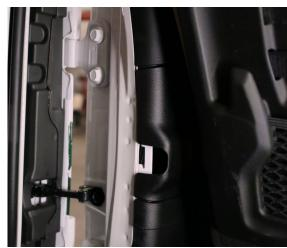
Use a T40 Torx Bit and remove the inner door catch.
