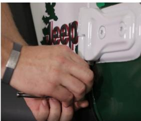
Remove the plastic cover. Push the red pin up to unlock, then pull the white lever upward as well.
