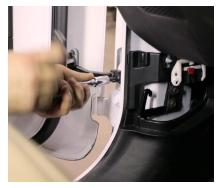
Remove the rear door. Begin with removing the plastic cover. Disconnect the wire by pressing inward on the clip. Bring the door inward so you can remove the doorstop. After you disconnect the wire and the door stop, put the plastic cover back on.
