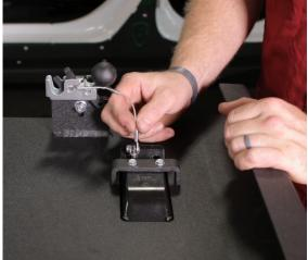
For the rear door, the hinges and the latch bracket will assemble the same way. Unlike the front door, the paddle lever will be on top. The latch opening will be mounted on top instead of being on the bottom like the front door. The lug attached to the cable should be facing the latch as shown in the picture below. Use a 1/8" Hex wrench to make sure its tight and doesn't move. On the paddle portion, the lug needs to swivel so make sure you do not tighten the nylock all the way.
