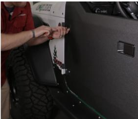
To adjust how far inward the door closes, adjust the latch on the inside of the door by loosening the button head bolts. If you make adjustments and notice the door is rattling, open the door back up and adjust the rubber door stop using a 3/16" Hex wrench.
