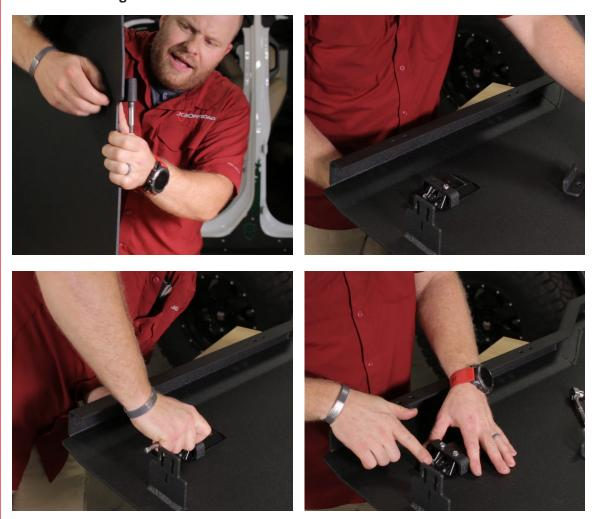
The level on the inside of the latch will be on top for the front doors and on the bottom for the back doors.
