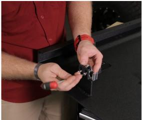
Next we will install the rubber bumper bracket. Press the rubber bumpers through the bracket in the orientation shown below. You may use a ball nose hex wrench or small screw driver to help get them through. Install the bumper bracket to the door using the supplied 5/16" button head and flange nut in the orientation shown below.
