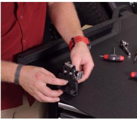
Next, connect the cable to the latch by inserting a button head bolt through the cable hole. Make sure the cable is pointed the same direction as the lever. Use a nylock to secure the bolt down so the cable doesn't move using a 1/8" Hex wrench.
