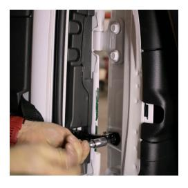
Assemble the door. Loosely install the hinges to the door so we can adjust them later. Mount the hinge to the door using a 5/16" button head bolt and a 5/16" flange nut. Use a 3/16" Hex to tighten the bolts. Next we will install the latch. Make sure the opening is facing forward. Place the bracket over the latch and secure the latch to the bracket using the self-threaded screws. Use a 8mm socket to tighten down the screws.
