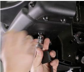
After you loosely reinstall the factory bolt into the support bracket, use a button head bolt and flange nut that we provide and secure the skid to the support bracket. Repeat these same steps on the otherside.
