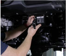
Next we will use the brackets that we have provided for you on the crossmember. Use a bracket, button head bolt, and a flange nut per side. Start by taking the flange nut and lining it up with the hole. Then line the bracket up with the hole and begin hand tightening the button head bolt. Make sure the bracket lines up with the edge of the crossmember. Once the bracket is lined up, use a 7/32 socket or hex end wrench to tighten the bolts.
