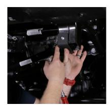
4 Next, take one of the factory torx bolts from the factory skid and bolt in the new skid. Use an extension for this part so you can run the bolt through the hole in the skid. Loosely bolt the factory bolt just enough to hold the skid up.
