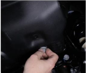
Remove the 2 bolts holding on the factory brackets using a 16mm socket. There are 2 bolts on each side on the inside of the frame crossmember. Once you remove both brackets, set them aside with the factory skid.
