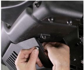
**6** With everything still loose, reinstall 2 more factory bolts that go up through the outer 2 slots of the skid. Loosely install these bolts with a T45 socket. After you install these bolts, go back and tighten down all of the bolts on the skid plate.
