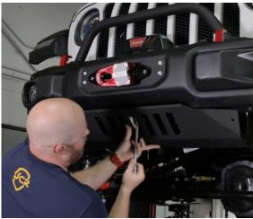
Take a button head bolt and flange nut that we provided and loosely install the skid to the bracket that we installed earlier. Next we will remove the outer 2 factory bolts on the bottom of the bumper to install the support brackets. Use a T45 socket. Once you remove the bolt, place the support bracket in place and reinstall the factory bolt that we just removed.
