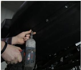
2 Next you will need to remove the trim plate. There is 1 snap fastener on each side of the frame rail to pop off with a flat blade screwdriver. After you remove the trim plate, disconnect the fog light harness on the passenger side as shown in picture C.
