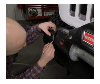
9 Once the winch is bolted down, reinstall the bumper. The winch will then be secured between the bumper and the factory framework.
