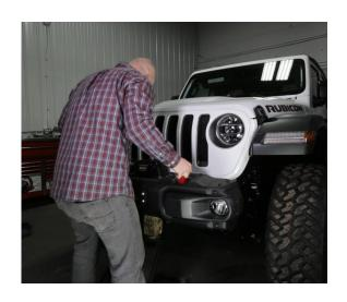
Next, tighten the bumper using the factory hardware. To tighten the inside bolts you may have to use an extension. Use a 5/8 socket to tighten the bolts we used earlier to hold the winch plate in place as shown in picture C and D.
