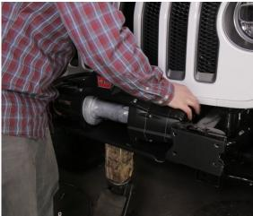
Next, remove the plastic blockoff plate on the factory steel bumper by pushing on the 6 clips holding the plate to the bumper as shown in picture A. Take the bracket that we provide and hold it on the outside of the bumper as shown in picture C. Bolt the bracket to the bumper with the button head hardware (4 bolts) provided in the kit as shown in picture D.
