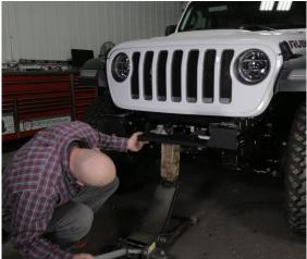
We have provided spacers that go between the winch and the winch plate. The spacers are meant to space the Warn Zeon upward so the freespool knob clears the top face of the bumper. If you are not using a Warn Zeon then you will NOT need the spacers. Bolt the winch to the winch plate with the bolts we have provided in the kit.
