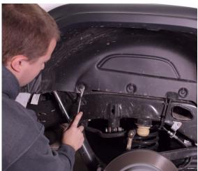
Use your dash tool to pry the inner fender away from the fender by pushing down and out. The only thing holding the inner fender in place are the clips between the inner fender and fender.
