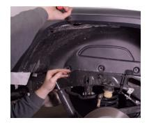
Next you will need to remove 2 of the upper fender clips (the 2 in the middle) and those will get replaced with the bolts we use for the inner fenders. Use your dash tool to remove these 2 clips. After you remove the 2 clips, make sure the other clips are secure to begin the install.
