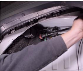
**6** Before we can install, we need to drill out the bottom 2 holes with a 5/16" drill bit. Once those are drilled we can begin installing the new inner fender.
