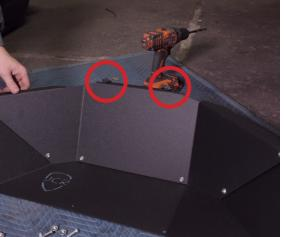
4 Now we will remove the stock inner fender. Start by removing the 8 Christmas tree clips holding the inner fender in place. There are 2 holding the lower left and right sides, 4 along the back, and 2 on top.
