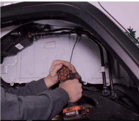
Next, use the longer 5/16" bolts to secure the top 2 bolt holes. Then secure 2 5/16" bolts in the bottom 2 holes with a flange nut on the back. Use a 3/32" allen to tighten these down along with the 4 bolts holding the 2 pieces together.
