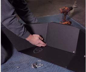
Next, install the 5/16" clip nuts to the 2 holes on top. Use your thumb to push these on over the holes.
