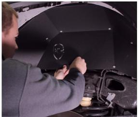
Use a 3/8 socket to secure the self-tapping screw to the bottom right hole. Once you install the screw, go back and make sure all of your bolts are tight then you can reinstall your wheel. Enjoy your new rear inner fenders!
