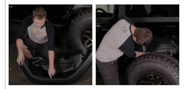
**3** Next, hold the inner fender up to the body to its approximate location then draw a line along the body with a marker. Leave part of the bump so you can mount the inner fender later. After you draw the line, remove the inner fender then cut along the line.
