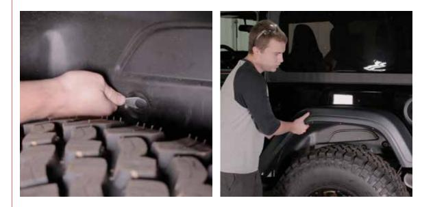
2 Once you remove the stock inner and outer fender, seperate them by removing the 8 plastic rivets using a 1/8" drill bit. After you seperate the inner and outer fender, reinstall the inner fender using 2 christmas tree clips.
