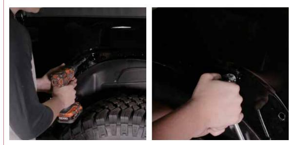
6 Next we will mount the fender. Using 2 5/16" button head bolts, mount the top 2 holes. Use the 1" long bolt provided in the hardware pack on the lower left hole. Use the 3/4" bolts for the rest of the holes. Use a 3/16" bit to tighten down all the bolts.
