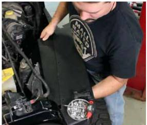
23 Make sure all wires, harnesses, and such are push out of the way before sliding the rear inner fender into place.
