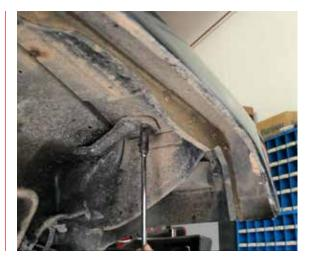
$\bf 3$  Continuing with the 13mm socket, loosen the top support bolts both at the grill and bulkhead.
