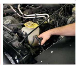
27 The Vacuum box gets relocated about 6 inches further in on the inner fender using the 1/4 button
