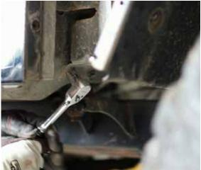
**14** Remove the 4 13mm bolts holding the fender to the body.
