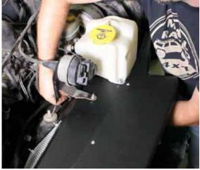
$26\,\,$  The horn on the driver's side uses the front perforated panel bolt to mount.
