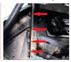
15 Track the turn signal and side marker wiring back to the grommet coming through the inside lower front of the fender. Push this grommet in so that it is no longer in the fender.
