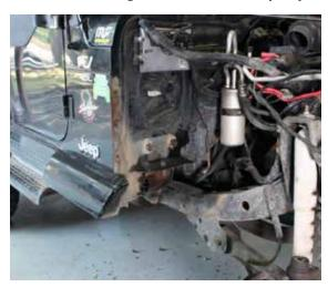
18 Install new battery tray bracket reusing three of the factory fasteners.
