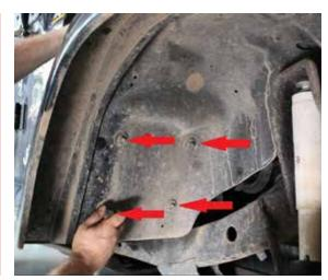
10 Remove the 6 bolts at the front of the fender into the grill. There are three on the back and three on the side.
