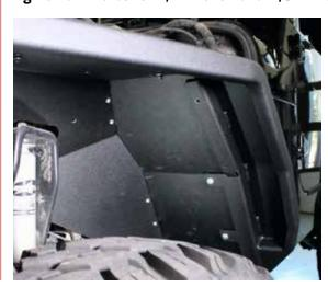
Install the accessories as show below using the 1/4 button heads and flange nuts.
