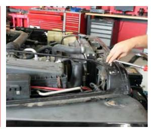
**4** Use a flat head screwdriver to unlatch the tabs holding the relay box. Some boxes will have 2 tabs, others will have 4.
