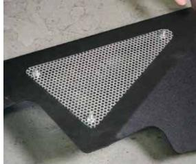
22 Slide the front inner fender panel into position above the shock tower and attach using the 1/4 button heads and flange nuts. Get them all started first and leave loose for now.
