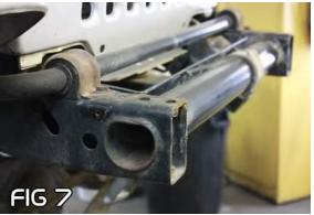
**5** Test fit your new JcrOffroad bumper to be sure that it properly fits over your frame, and that all mounting holes align properly.
