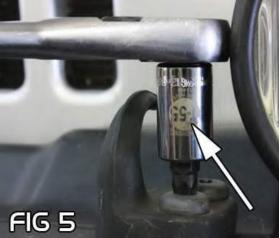
4 Remove the lower bumper bolts with a T55 torx socket (fig 6).
