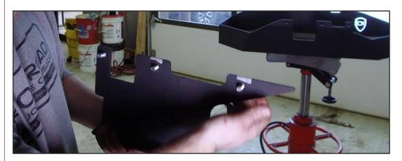
To ensure that the bolts are not lost or fall into the skid during install, we recommend using some masking tape on the back of the bolts.
