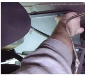
**3** Using a C -Clamp, clamp the flat edge of the factory gas tank skid to the rear cross member in a spot that will allow access to the factory gas tank skid nuts.
