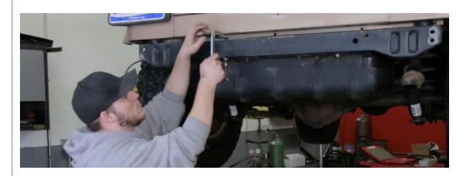
4 Loosen the front factory gas tank nuts using a 1/2" socket or wrench. If using a socket, an 11" extension may make this process easier.
