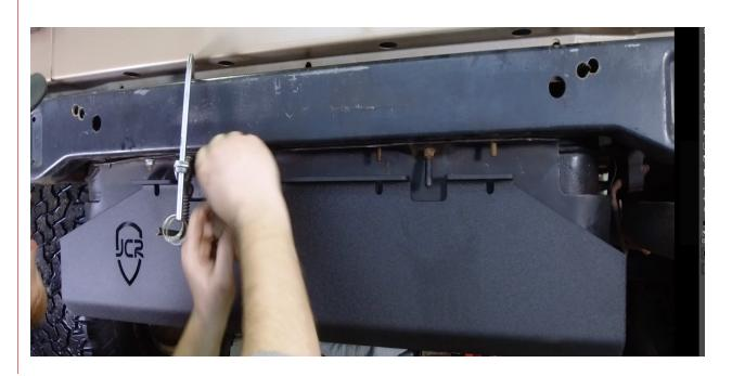
**8** Lift the new skid into place. Replace factory nuts and tighten. Go back and completely tighten all of the bolts. To make sure everything tightens evenly, work front to back.
