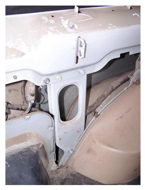
Now, hold up the LQG to the Jeep good and tight and mark the upper center hole. Set the LQG down and drill a 5/16" hole. Apply a small bead of RTV or silicon to the back of the guard being sure to make it around each bolt hole and the perimeter of the guard. Mount the LQG using the hole you just drilled. This will be enough to hold the weight of the LQG while you drill the rest of the holes.
