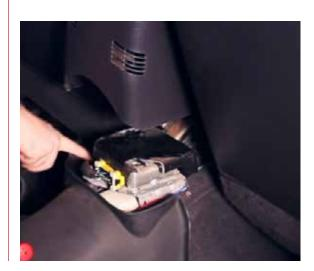
Remove the three Phillips head screws holding the stock center console to the body. There is one in the front on the passenger side, one on the rear on the passenger side, and one on the rear drivers side. Remove the stock bracket and any broken pieces once it is free.
