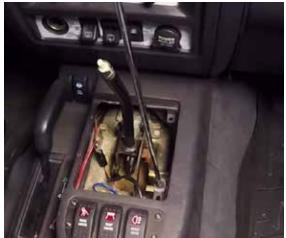
4 Remove the four wheel driver selector bezel, this may need a flat tool to pry up. Now use a Phillips head screw driver to remove the screw in the middle near the selector.
