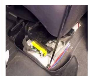
Place the new JcrOffroad center console bracket into place. Make sure that the side with one leg goes in facing forward, like the photo below. Start to thread all three mounting screws in before tightening them down.
