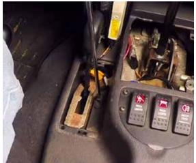
Moving to the back seat, you can now lift the center console up to see the broken stock center console bracket. You should be able to wedge the center console between the seats to hold it up.
