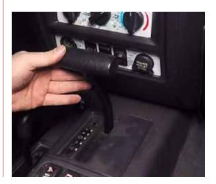
Remove the shifter bezel, you may need a flat tool to pry up. Watch for the light on the divers side that will need to be unplugged to remove the bezel. Now use the Phillips head screw driver to remove the screw in the lower right corner of shifter opening.
