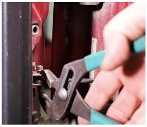
Next, remove the torx bolts from the door. Remove 5 of the 6 bolts on the bottom while leaving one bolt on the top. We recommend you have a friend hold the door for you while you remove the 6th bolt on top so the door does not get damaged.
