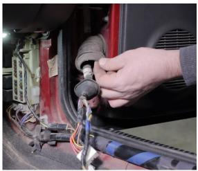
Be very careful when pulling the wires through the door. Do not tug on the wires as they may become loose or separate.
