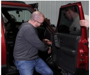
Repeat steps 1-5 for the back doors. Remember to remove the panels, disconnect the wires leading into the door, and then removing the pin that holds the door stop in place. Before removing the torx bolts from the hinges, close the door and loosen the bolts from the opposite side as shown in the picture below. Then, you may repeat the steps used in removing the front door.
