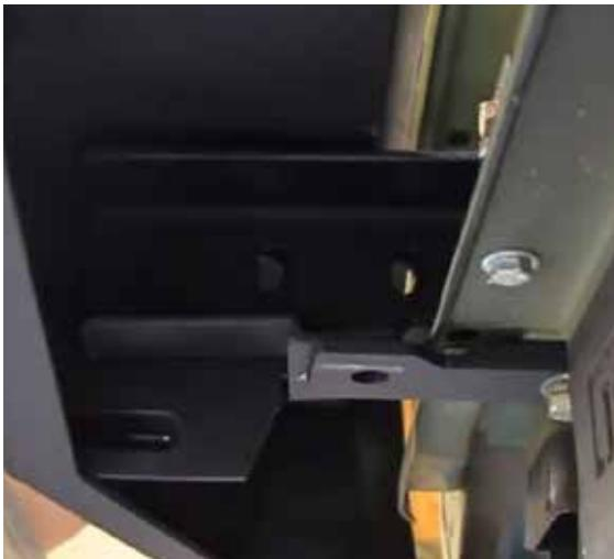
**13** Adjust bumper pitch and height with the 5/8" bolts, or left and right with the frame side bolts/slots. Check the operation of the tailgate, lower the bumper down if the gate hits the top of the bumper.
