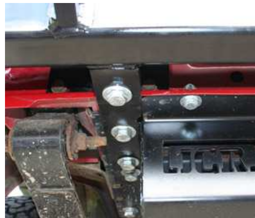
Lower Tie-in bracket installed.
