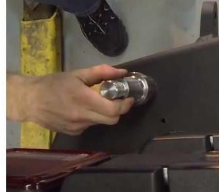
3. With the spindle in the bumper, install the lower 3/4" grade 8 bolt into the bottom of the spindle. You may need to lift the spindle a little to help get the bolt threaded. Once you have the bolt started use a 1 1/8" wrench to tighten the lower bolt.
