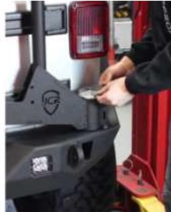
8. Install the plunger into the threaded mount next to the hub assembly.
