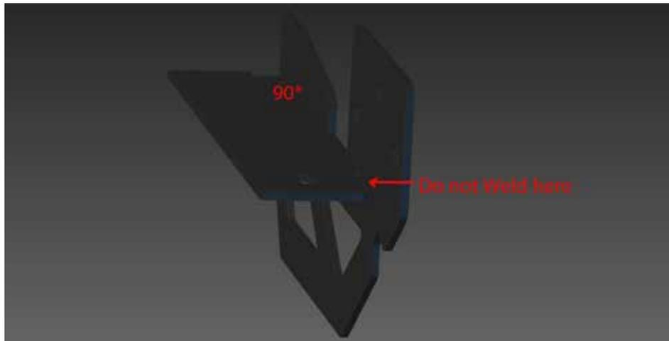
**5** With everything bent, it's time to start tacking everything together. It's best to weld and grind the shell of the bumper without the Dring tabs or Bumper mounts welded on first.
