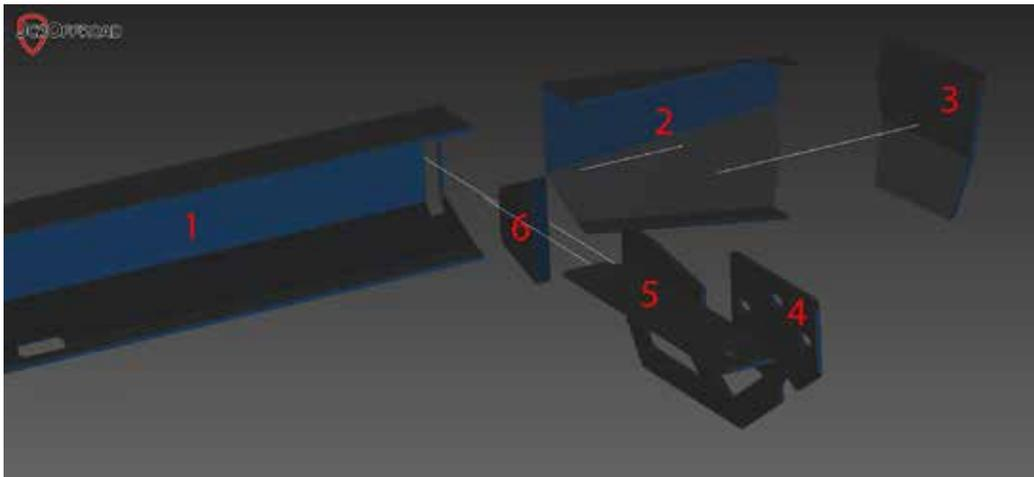
**6** With the bumper Welded and ground, install the Dring Tabs (6) through the bumper from the back. The Tab will stick out the back about 1/2". Tack weld on the inside of the bumper, as the Bumper Mount will mount flush against the outside of the tab.
