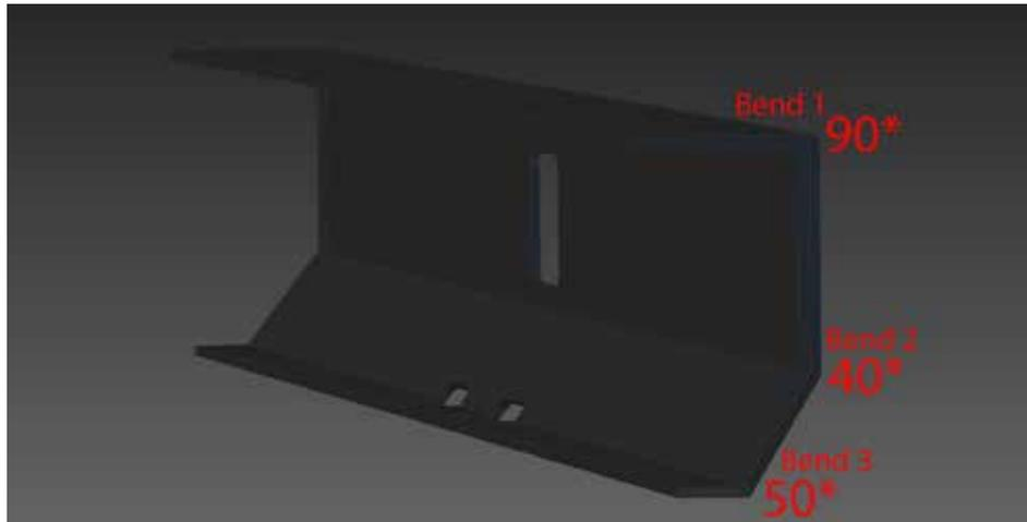
**2** Set the bent Center Section (MJDIY01) off to the side. Next you will need to bend the two Bumper Wings (MJDIY02). **\*\*\*You will need to bend a Right and Left, which will end up having two wings that are opposites.\*\*\***
