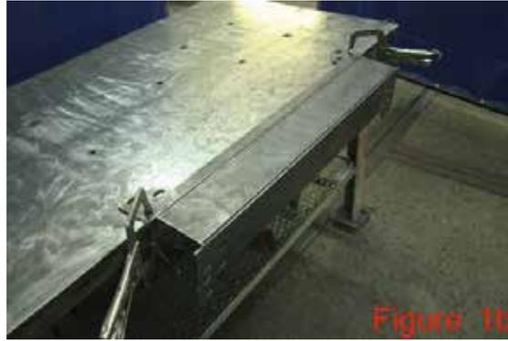
**2** Set the bent Center Section (1) face down on a table, verify the inside width at the mounts to be 4-1/8" on both sides. After the Center Section has been correctly bent, you can set it off to the side until later in the assembly process. (shown in figure 1c)
