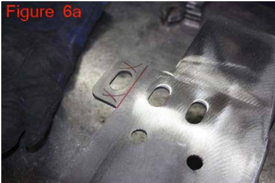
**9** Mounting on a Jeep YJ. The lower tab will need to be trimmed to allow for clearance with the front leaf spring shackles. The area needing trimmed is pictured in Figure 6b.
