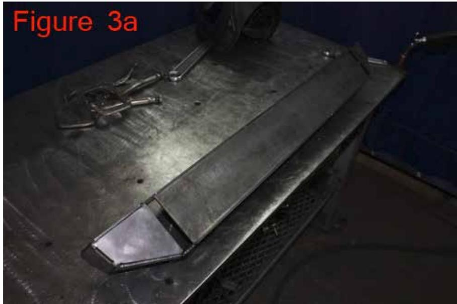
**4** With the bumper tacked together, it is now time to fully weld the bumper together. We recommend welding the back side first.
