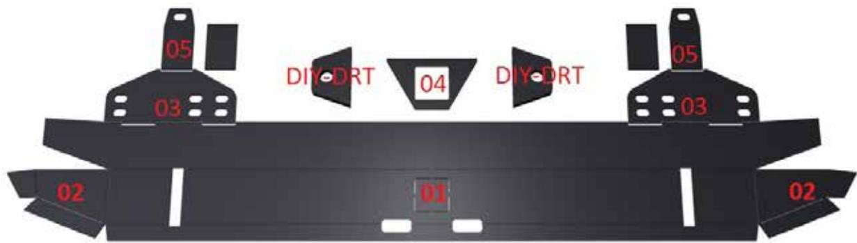
**1** The first piece you will want to bend will be the (01) front Center Section. You will be bending two 90\* angles. It doesn't matter which side you make the front.
