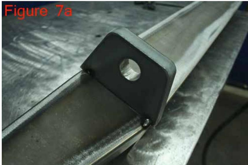
Setting up the Mounts for TJ/YJ or CJ. These kits are designed to work with a TJ, YJ or CJ. Included in this kit are universal mounts that will fit both TJ/YJ and CJ. Look very carefully at the diagram below to see how to properly set up your DIY bumper to fit your Model Jeep.
