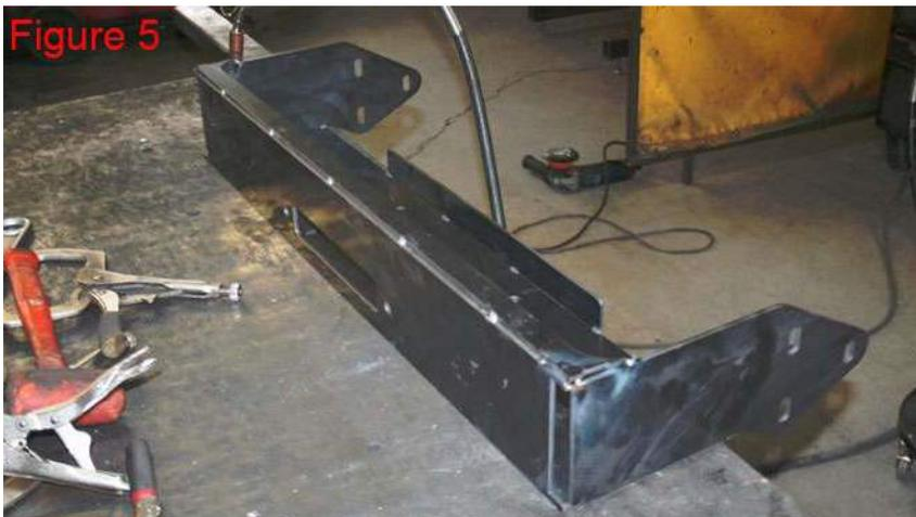
**6** With the center of the bumper tacked together, you will now tack on the outer Wings (3)
