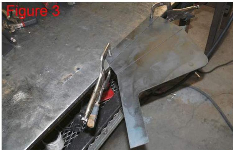
**4** You will now be bending the two Side Protection parts (4). The long angle will be bent to 65° and the small back flap will be bent over to butt against the other bend.
