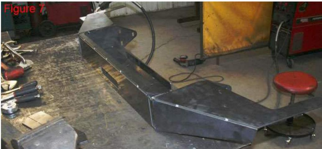
**8** The next parts to be tack on will be the Side Protection caps (4). Clamp the caps to the bumper and tack weld each side (Figure 8)
