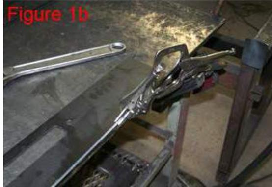
**2** Set the bent Center Section (2) off to the side. Next you will need to bend the Winch Plate and Mounts (1) There will be three bends, all will be bent to 90°.
