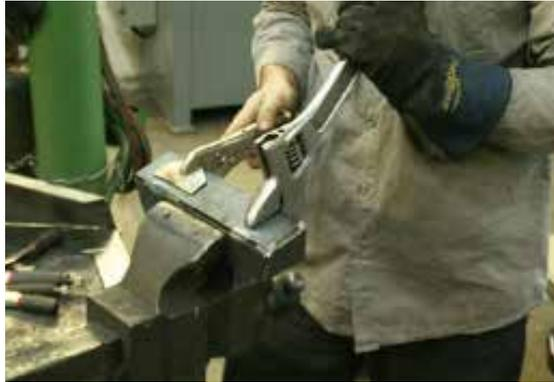
**4** The next parts to be bent will be the filler caps for under the tail lights, part #4. **\*\*\*You will need to bend a Right and Left, which will end up having two caps that are opposites.\*\*\***
