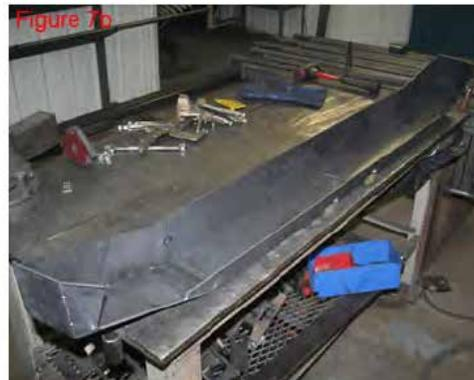
**9** With the shell of the bumper tacked together, it's now time to weld it completely.
