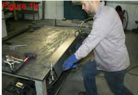
**2** Set the bent Center Section (1) off to the side. Next you will need to bend the two Bumper Wings (2). The Top bend will be at 90\* and the bottom at 40\*. \*\*\*You will need to bend a Right and Left, which will end up having two wings that are opposites.\*\*\*
