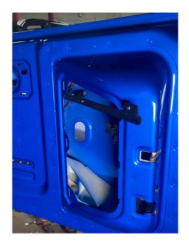
Once both nut strips are into the tailgate, bolt them into place using four 1/4"-20 X 3/4" button head bolts with one of the larger 1/4" USS washers on each. Bolt them into the holes circled in red below. Try to center the bottom nut-strip as well as you can before tightening it into place.
