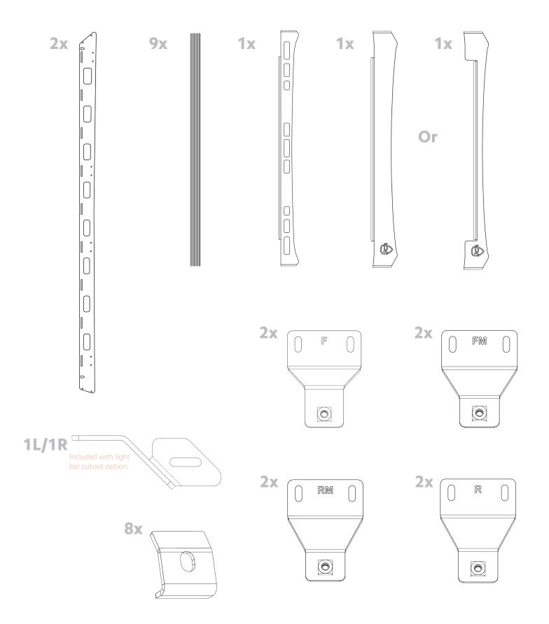
Assemble the rack on the ground. Start by mounting the crossbars between the 2 side rails. For this, use the1/4"-20 X 3/4" button head bolts and the 1/4" ID washers (2 per bar per side). Make sure the machined slot in the rail of the crossbar is facing up, so that you can easily add t-nuts to mount your gear.
