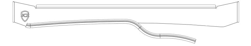
3 Next, mount the front and rear fairings. To do this, use the1/4"-20 X 3/4" button head bolts, 1/4" ID washers, and 1/4"-20 serrated flange nuts. The front fairing will need 2 of each per side and the rear fairing will also need 2 of each per side. When mounting the front fairing, adjust it all the way up to avoid contact with the roof and leave the bolts loose enough to be able to make adjustments once it is on the roof of the vehicle.
