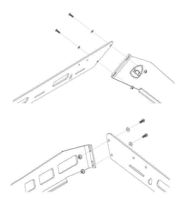
4 Next, loosely attach the inner mounts to the inside of the side rails using the 1/4"-20 X 3/4" button head bolts, 1/4" ID washers, and 1/4"-20 serrated flange nuts. The order that the mounts go on from front to rear is F, FM, FR, R. Make sure that the side with the square nut on it is facing out, away from the vehicle.
